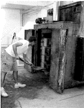
Figure 3: An industrial oven was used to remove moisture from the sand used in the dry soil layers.
